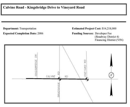
This project is to widen Calvine Road from two to four lanes between 1,000 feet east of Kingsbridge Drive and Vineyard Road. The project will also include bridge widening at the crossing of Laguna Creek and the installation of signals at Bradshaw Road at Calvine Road; Calvine Road at Vineyard Road; Grant Line Road at Calvine Road; and Calvine Road at Bader Road, a 12-foot wide landscape median and paved shoulders. This project includes improvements within the City of Elk Grove.
