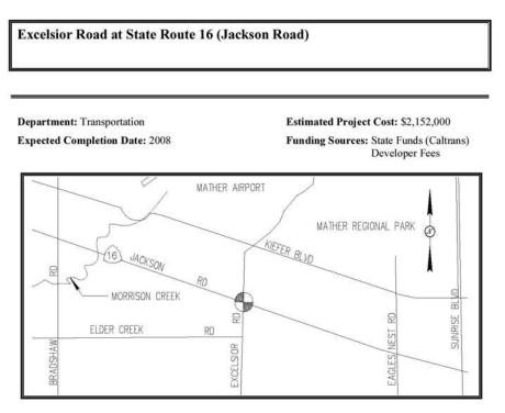
This project will install a traffic signal at the intersection of Excelsior Road and State Route 16 (Jackson Road) and minor widening with restriping to accommodate separate turn lanes with multipurpose lanes. The State Department of Transportation (Caltrans) will be administering the project with a cooperative agreement with Sacramento County to help fund this project.
