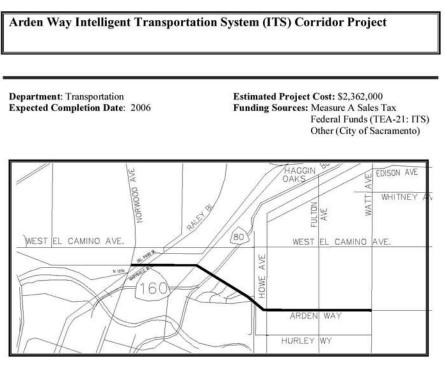
The City of Sacramento is in collaboration with the County of Sacramento's plan to install various Intelligent Transportation System (ITS) elements along Arden Way between Watt Avenue and Del Paso Boulevard. As part of the Arden Way ITS, the proposed ITS elements will work to improve traffic management and mobility along Arden Way and provide a communication link between the city and county communication hubs.
